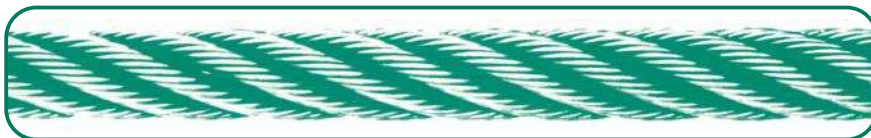
RIGHT HAND REGULAR LAY ROPE (sZ)
